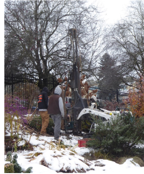
Geotech company measuring ability of the soil to absorb water (Left), Drilling to measure weight bearing capacity of soil (Right)
